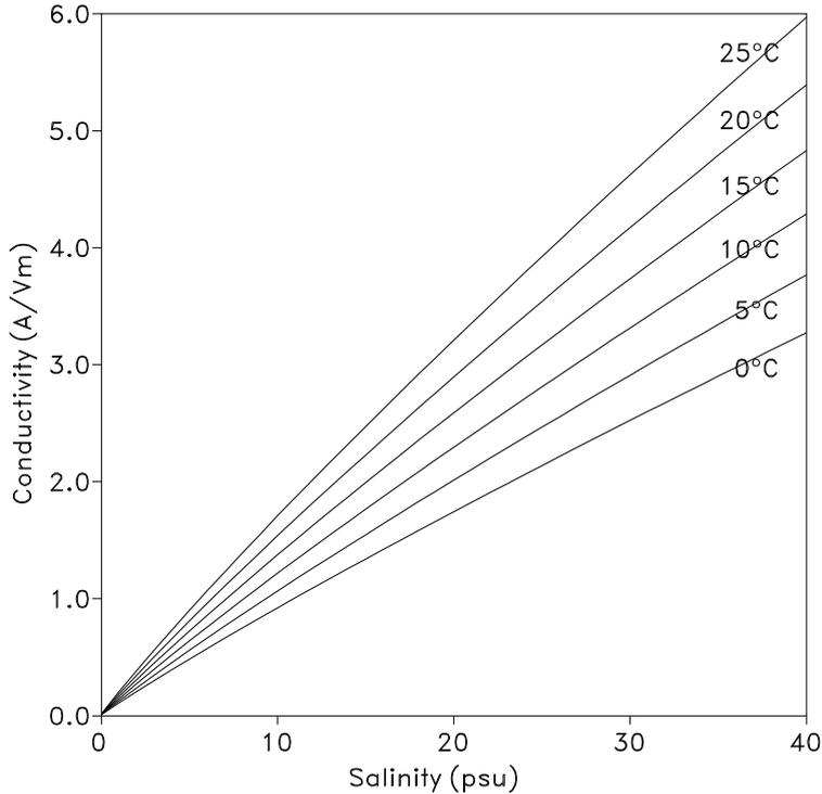
Figure 1. Conductivity of sea water as function of salinity at six different temperatures.
