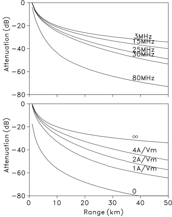
Figure 2. Theoretical HF attenuation (arbitrarily normalized) over a plane ocean. Upper panel: in terms of frequency at a conductivity of 4 A/Vm (ocean water, cf. figure 1), lower panel: in terms of conductivity at a frequency of 25 MHz.
