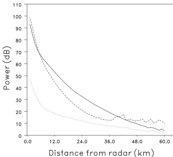
Figure 5. Signal strength versus range, as measured by the HF radar WERA. Full lines refer to a mean wave height of  $H_{1/3} = 60$  cm, dashed lines to  $H_{1/3} = 400$  cm. Dotted line displays the system's internal noise which is independent of sea state.
