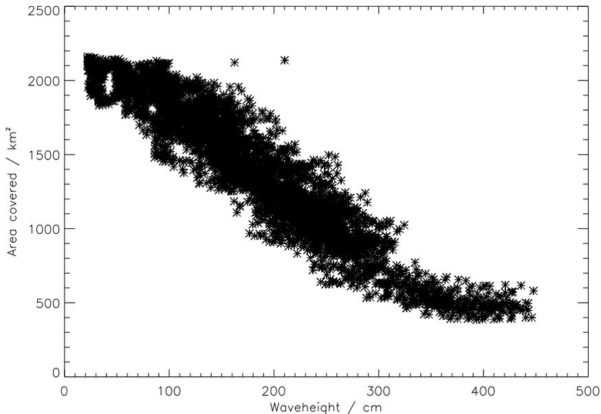
Figure 6. Area covered by two separate HF radars as function of mean waveheight ( $H_{1/3}$ ). Coverage of a grid patch is established if both radars reveal a significant first-order signal.
