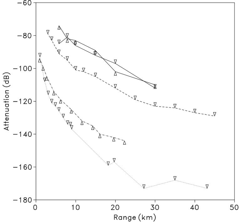
Figure 3. Measured HF attenuation at different sites. Full lines: North Sea ( $\sigma = 4.0$  A/Vm), dashed line: Baltic ( $\sigma = 1.5$  A/Vm), dashed-dotted line: fresh-water lake, dotted line: ice. The transmit frequencies are 25.25 MHz ( $\nabla$ ) and 29.85 MHz ( $\triangle$ ).
