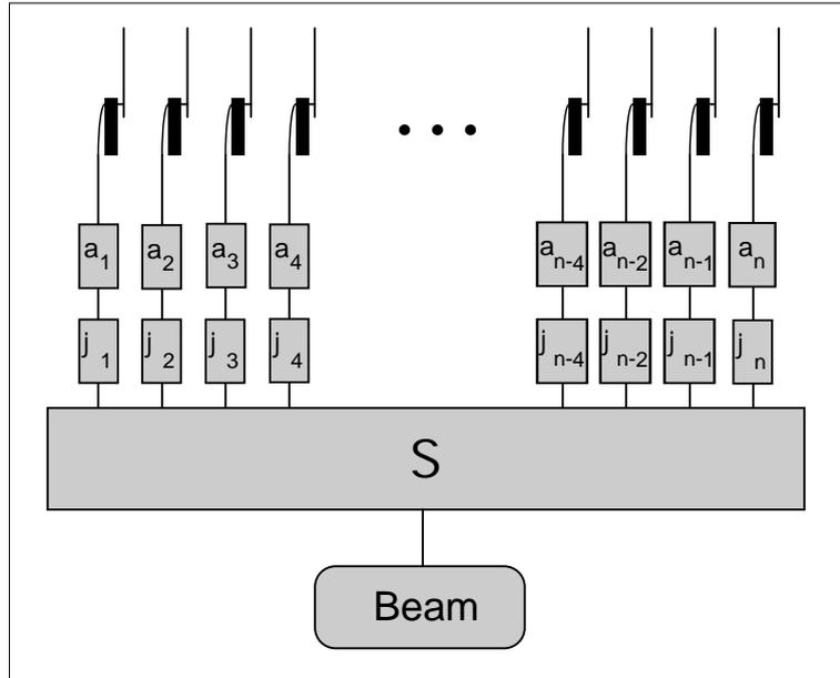
Figure 10. Principle of beamforming. After weighting by  $a_i$  and phase shifting by  $\varphi_i$  the signals of  $n$  receive antennas are added.
