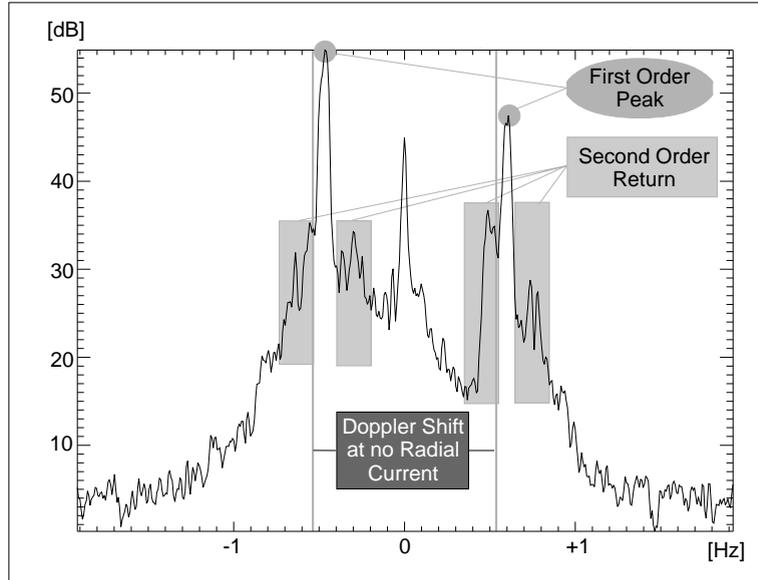
Figure 4. Measured HF Doppler spectrum. First-order lines and second-order side bands are indicated.
