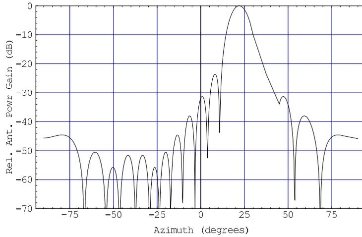
Figure 11. The theoretical antenna pattern of a 16 element array when the beam is steered  $22^\circ$  off boresite. Cosine weighting has been applied in this case.
