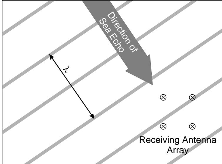
Figure 9. Principle of direction finding. The diagonal of the square antenna array is  $1/2$  of the electromagnetic wavelength  $\lambda$ .
