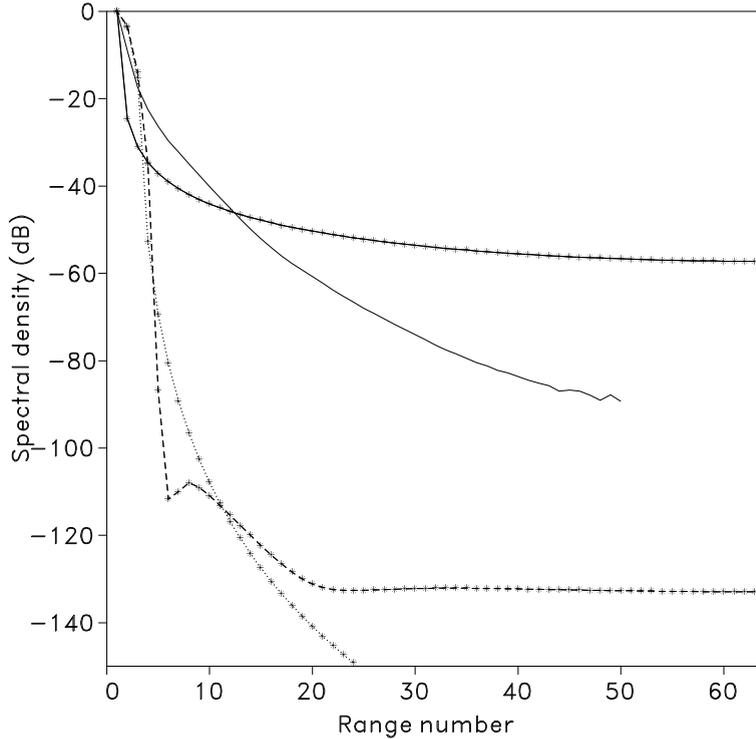
Figure 8. Spectral density of a synthesized chirp, applying no window (solid line with stars), a Blackman-Harris window (dashed line with stars) and a  $\cos^4$ -window (dotted line with stars). The solid line reproduces the measured signal strength of figure 5.
