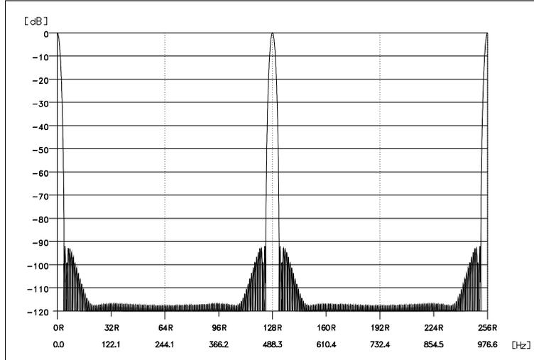
Figure 7. Filter function of 128 CODAR samples, weighted by a Blackmann-Harris window.
