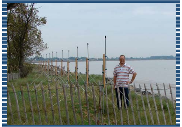
VHF receive array with 12 antennae near Nantes
