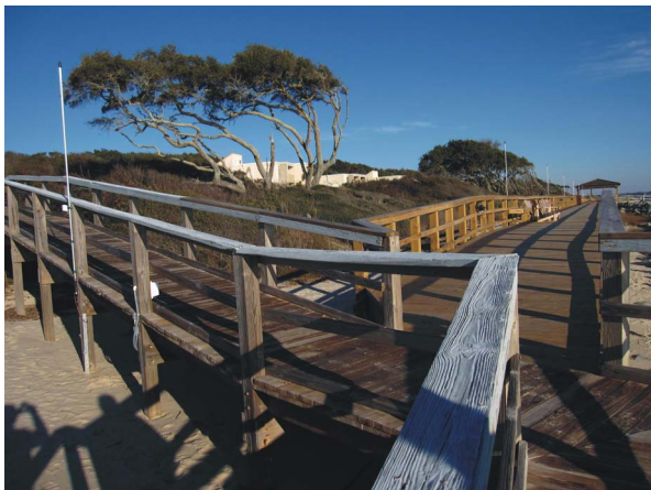
Figure 1. WERA antenna array integrated in a boardwalk at the coast of Georgia, USA (photo provided by Dana Savidge, SKIO)
