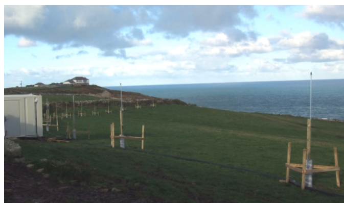
Figure 2. Curved WERA receive array on a ranch in Cornwall, UK, with "bull proof" antennae for 12 MHz. The simple monopole antennae are 2.5 m in height and stable without any guy ropes
